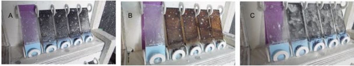
Figure 3: Comparative images of the type A, B and C hybrid films from the video taken during the simulated freezing rain test ( -18^{\circ}\text{C} )
